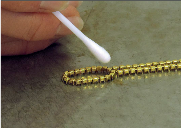
1. Degrease and dry the underside of the metal setting(s).
